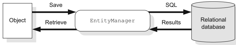
Figure 10.1 The EntityManager acts as a bridge between the OO and relational worlds. It interprets the O/R mapping specified for an entity and saves the entity in the database.
