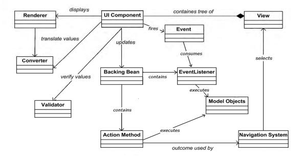
This simplified UML class diagram shows the different concepts of JSF.
