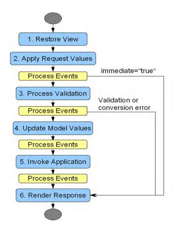
When a JSF view is requested, the components in the view are asked to perform tasks in a certain order, defined as phases of a request processing life cycle.
