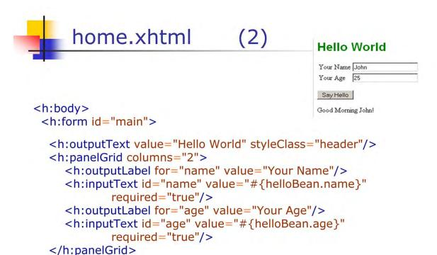
The <h:form> tag represents an HtmlForm component, which is a container for other components and is used for posting information back to the server. We can have more than one HtmlForm on the same page, but all input controls must be nested within a <h:form> tag.
