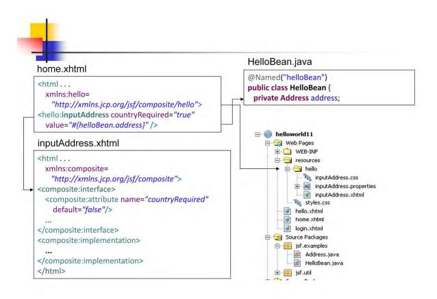
Here we can see the different parts which are necessary to build a custom component and their dependencies.
