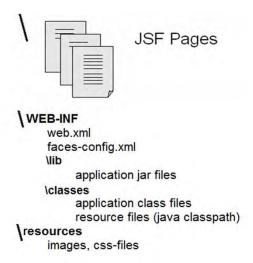
Because JSF applications are standard Java web applications, all of the necessary files must be packed in a directory structure that can be deployed to the web container. For JSF applications, there are two additions: the faces-config.xml file (where certain JSF configurations are placed) and (if your web container doesn't already support JSF) the JAR files of your JSF implementation. The resources directory contains resources like images or css style sheets.
